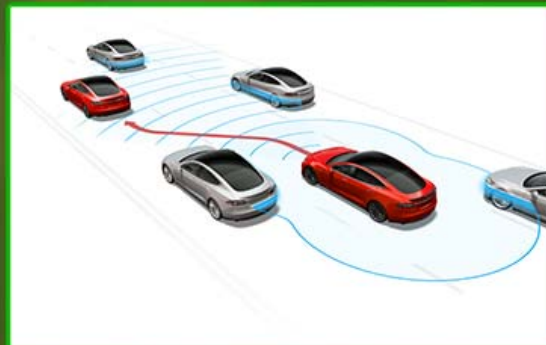
A visualisation of how a Tesla senses its environment and performs a lane change
