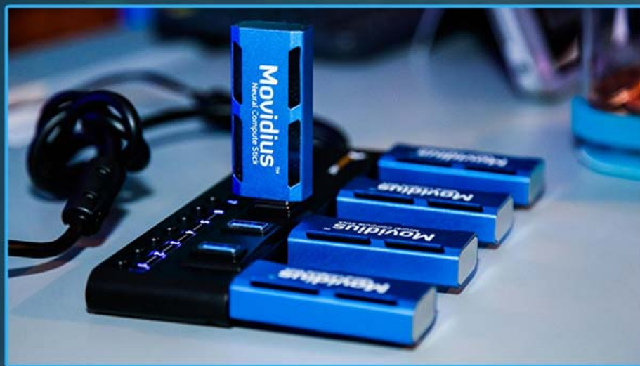
Although a single stick is typically used, people have created Intel Movidius neural compute stick clusters
